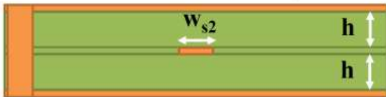
Cross-section of 3-layer stripline
