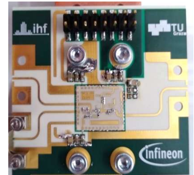
Doherty PA module in testboard
